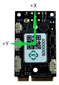
Both the Point One Standard Dev Kit and the GNSS antenna must be mounted **rigidly** to the vehicle. You must specify the rough orientation of the device relative to the vehicle, and then the device calibration procedure will estimate any differences between the device mounting angles and the vehicle axes.
