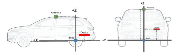
Once installed, you must measure the lever arms from the vehicle body frame to both the device and the GNSS antenna. For best performance, it is important to measure the lever arms as accurately as possible, ideally to better than 5cm of accuracy. The following lever arms may be specified:
